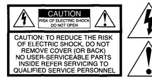
This symbol warns the user that uninsulated voltage within the unit may have sufficient magnitude to cause electric shock. Therefore, it is dangerous to make any kind of contact with any inside part of this unit.
