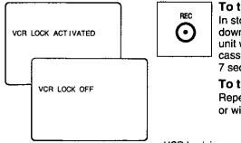
**To turn "ON."** In stop mode, hold down REC on the unit without a cassette inserted for 7 seconds.
