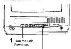
${f 2}$  Press and hold both PLAY and FF on the unit for more than 5 seconds. The power will shut off.
